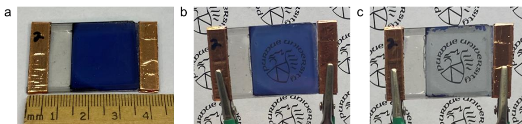
Supplementary Fig. 14. Photographic images of ECP-B ECDs with n -PBDF electrodes for size confirmation (a), in colored (b), and bleached states (c).
