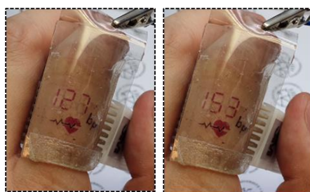
Supplementary Fig. 50. Photographic images of operation of all-polymer segmented electrochromic display on human finger (bending radius = 1.5 cm).
