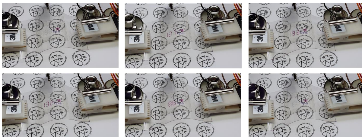
Supplementary Fig. 49. Photographic images of operation of all-polymer segmented electrochromic display in bended condition.
