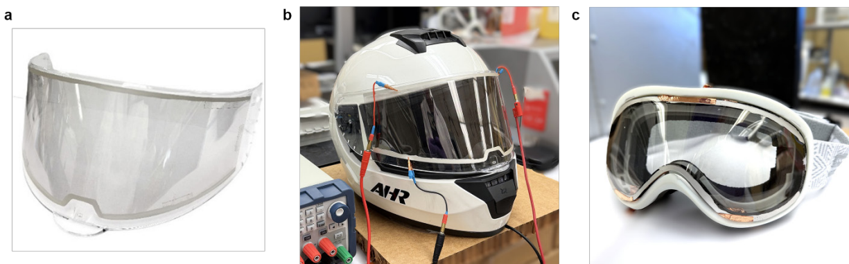
Figure S39. Flexible n -PBDF transparent heaters and demonstration of practical applications.
